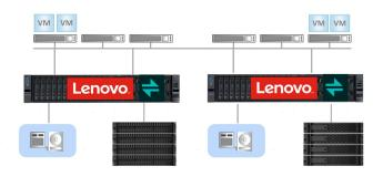
The Lenovo SDS Solution with DataCore allows you to unify, virtualize, and manage heterogeneous storage. Data services can be propagated across all storage arrays and the solution can be scaled up or out by adding more capacity or more virtualization nodes.
