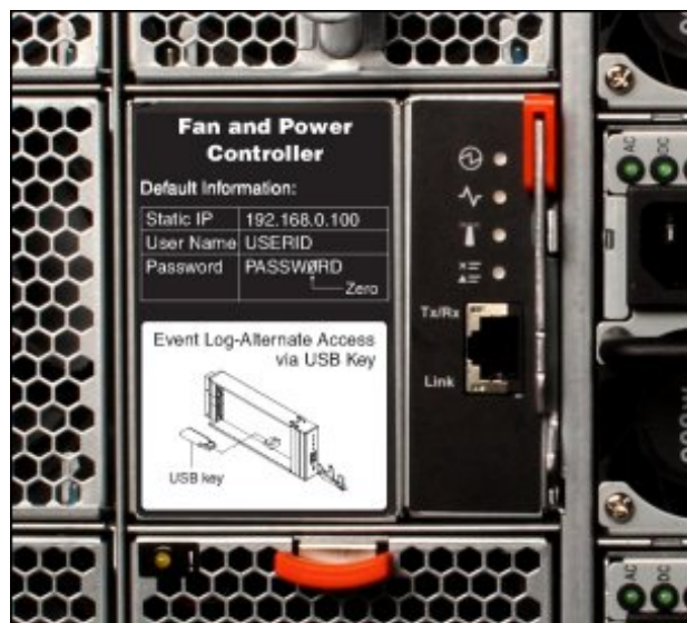
Figure 18. Fan and Power Controller
