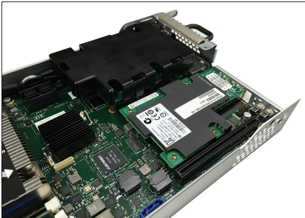
Figure 10. Adapters installed in front of the sd350
