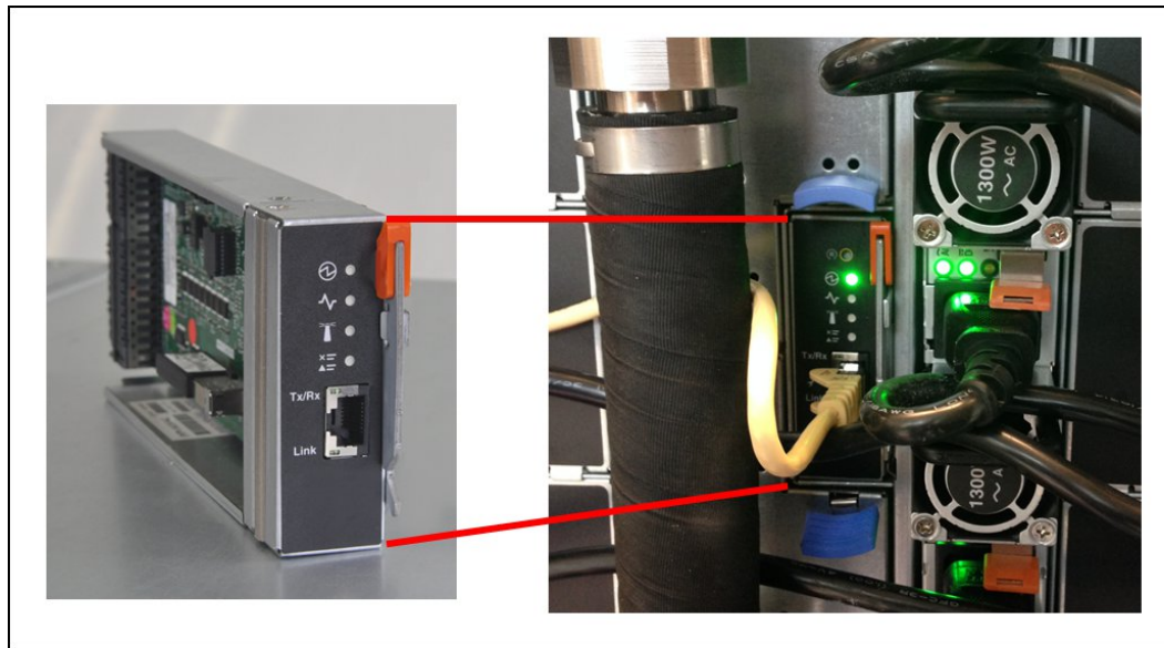
Figure 11. Fan and Power Controller
