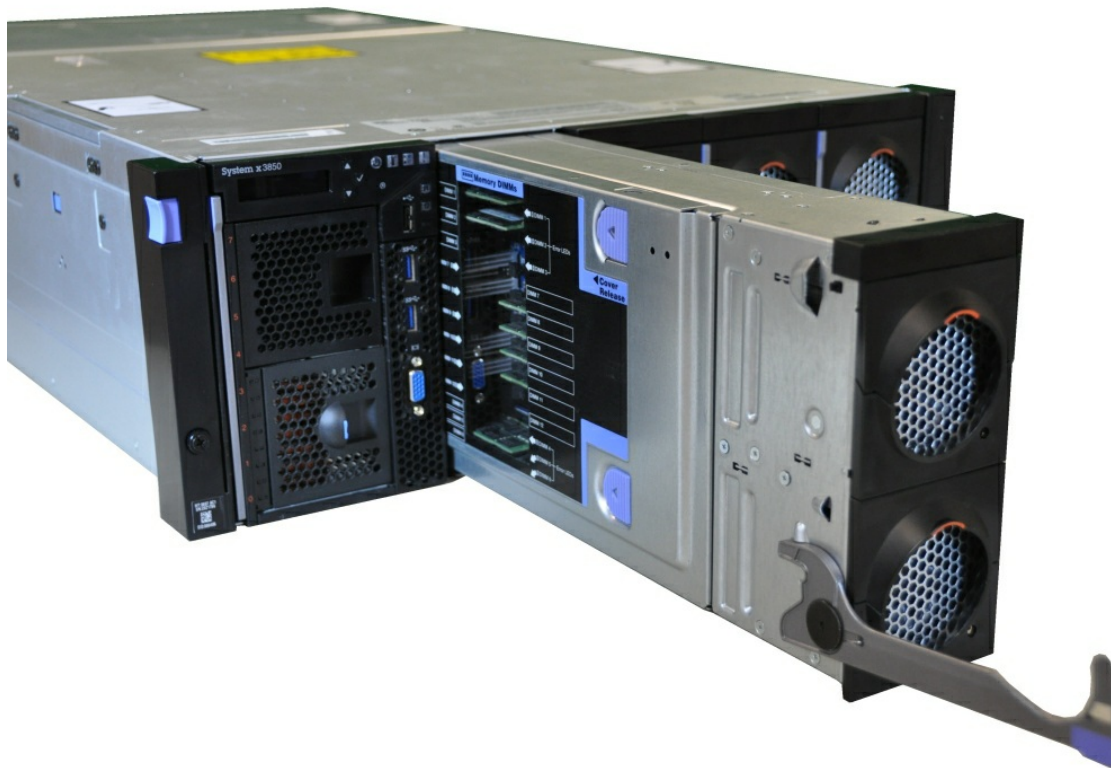
Figure 3. The X6 servers make servicing easy because components like the Compute Book are easily removed from the front or rear of the server
