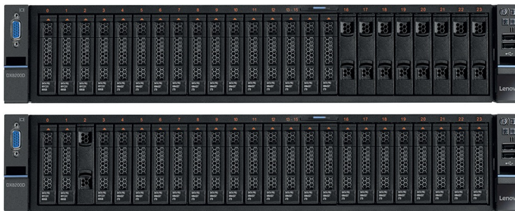
Figure 1. Lenovo Storage DX8200D models: Storage Virtualization (top) and ServerSAN (bottom)
