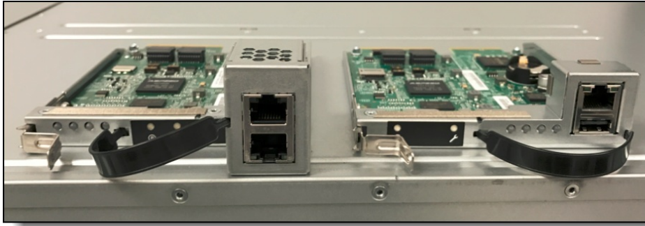
Figure 18. Dual-port SMM and standard (single-port) SMM
