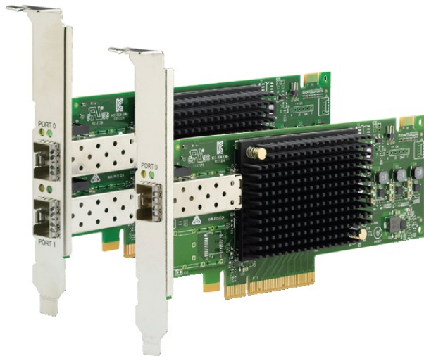
Figure 1. Emulex 32 Gb Single-port and Dual-port HBAs (shown without the included SFP+ modules)
