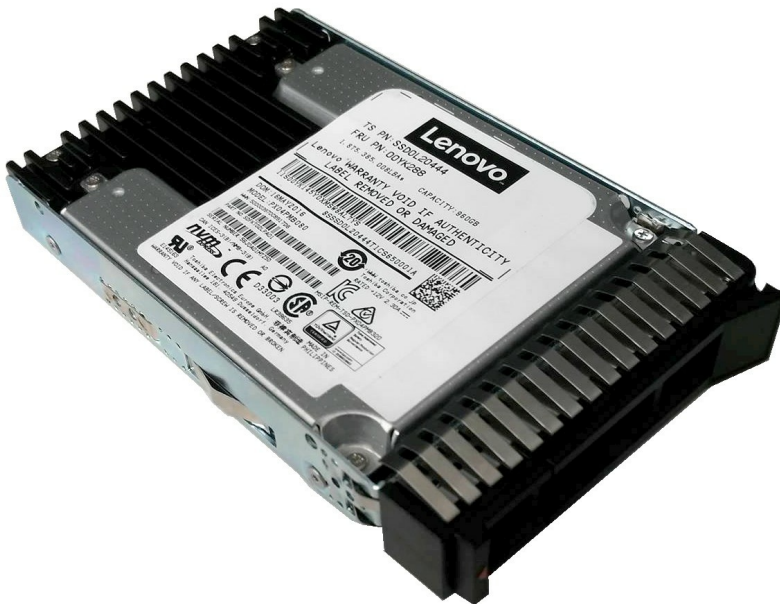
Figure 1. Lenovo PX04PMB NVMe Performance PCIe 2.5-inch SSD
