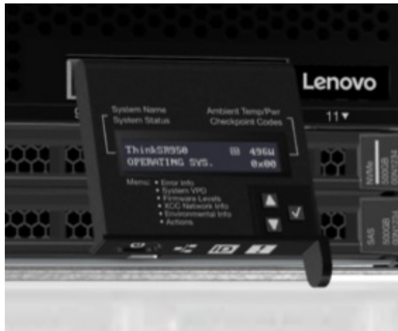
Figure 8. LCD pull-out display panel
