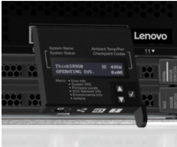
Figure 8. LCD pull-out display panel
