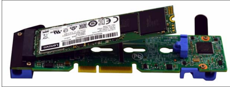
Figure 2-28 Dual M.2 Boot Adapter and a 128 GB M.2 drive
