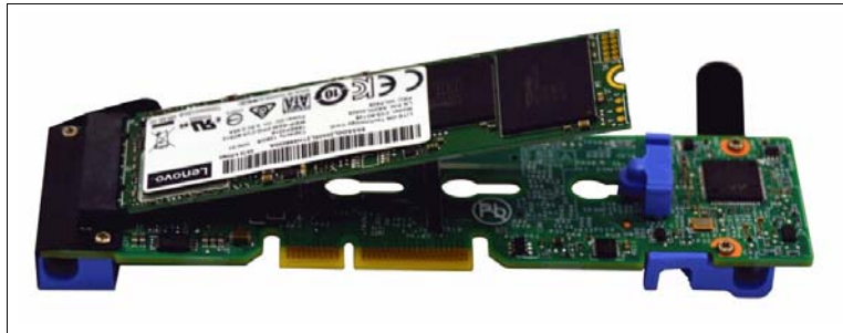
Figure 3-13 Dual M.2 Boot Adapter and a 128 GB M.2 drive
