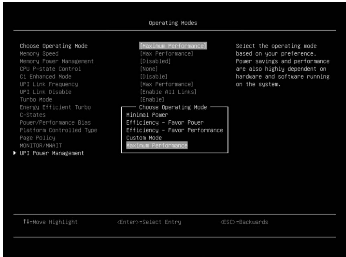
Figure 13 Operating Mode in UEFI menu
