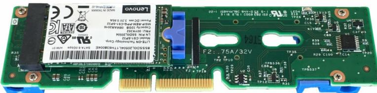
Figure 6. Single M.2 Adapter and a 32 GB M.2 drive
