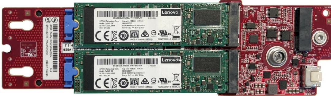
Figure 4. SATA/NVMe M.2 Module with 2 drives
