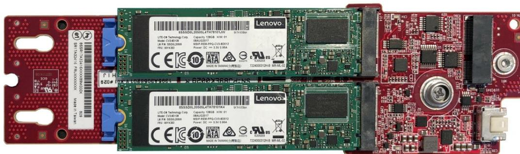
Figure 4. SATA/NVMe M.2 Module with 2 drives
