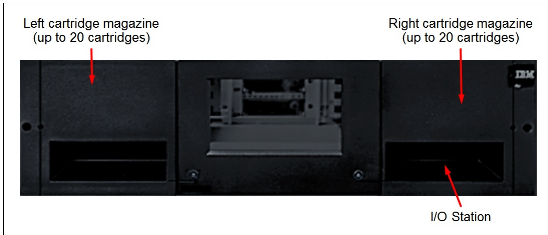
Figure 3. Front view of the TS4300 Tape Library expansion module
