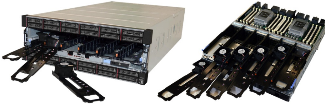
Figure 3. The fans are close to the processors but still front-accessible for hot-swap removal
