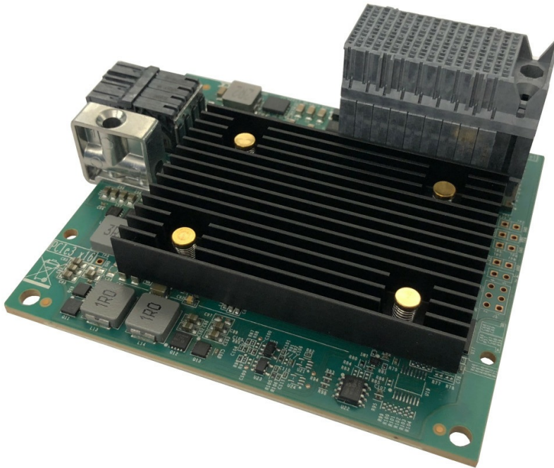
Figure 1. QLogic QL45000 25Gb and 50Gb Flex Ethernet Adapters (QL45214, QL45212 and QL45262)
