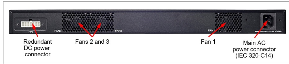
Figure 9. RackSwitch G7052 non-port-side view
