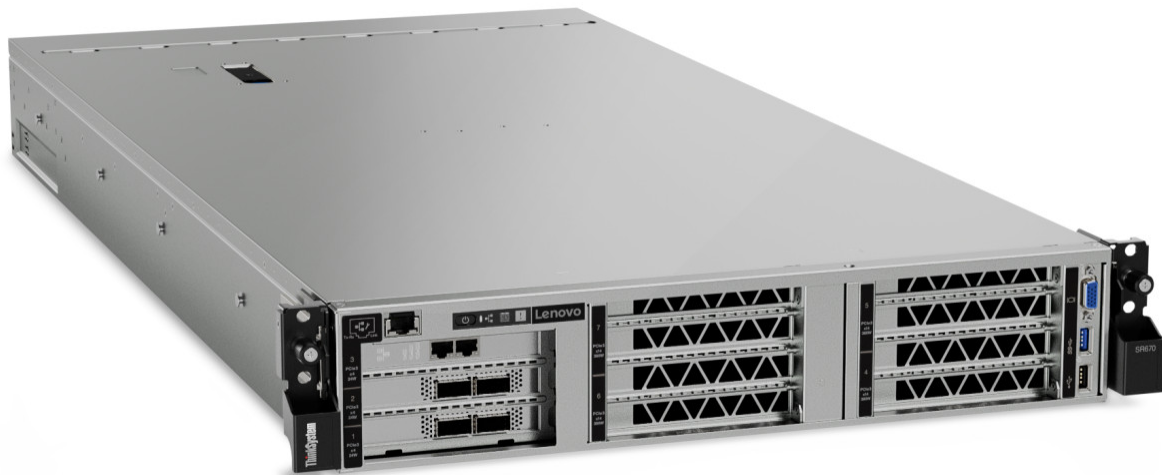
Figure 1. Front view of the Lenovo ThinkSystem SR670
