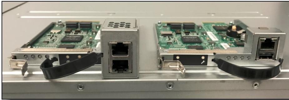
Figure 18. Dual-port SMM and standard (single-port) SMM
