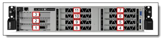
Figure 9. Location of the PCIe slots (front of the server) - eight single-wide GPU slots
