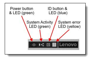
Figure 10. Front operator panel
