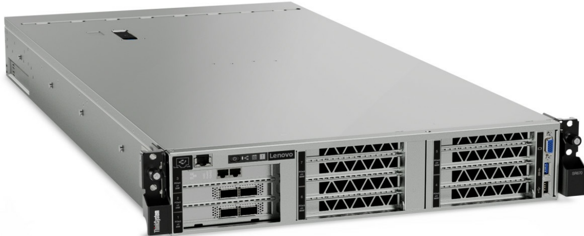
Figure 2. Front view of the Lenovo ThinkSystem SR670
