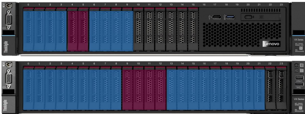
Figure 6: ThinkAgile VX650 V3 node with 2 OSA disk groups of one cache drive and 4 capacity drives ThinkAgile VX850 V3 node with 4 OSA disk groups each with one cache drive and 4 capacity drives
