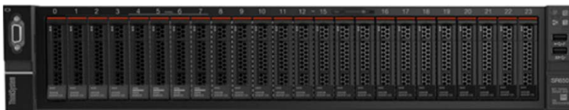
Figure 4. Lenovo ThinkSystem SR650 (with 24 x 2.5-inch disk bays)
