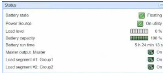
Figure 29 UPS information panel
