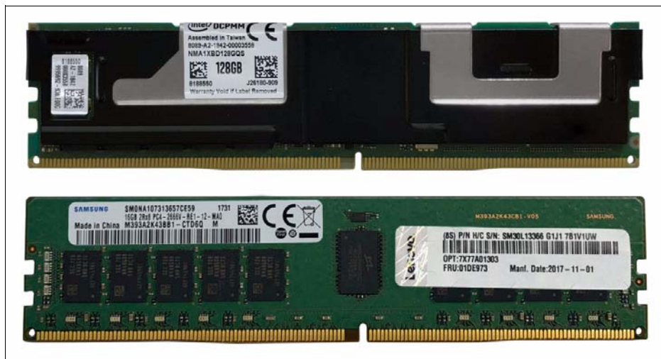
Figure 1 DCPMM (top) and a DDR4 RDIMM (bottom)
