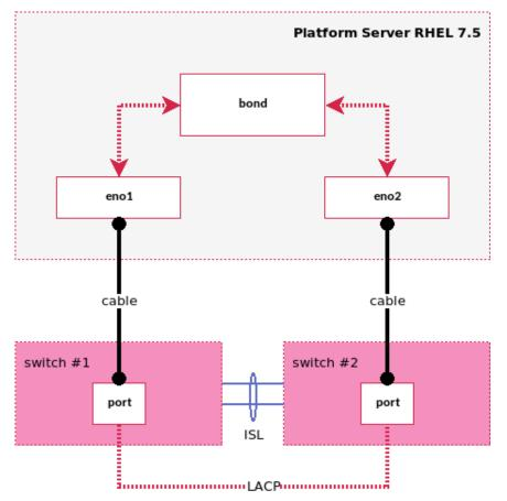
Figure 15: Network connection for servers and switches.
