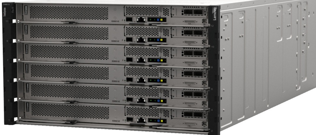
Six servers in a 6U enclosure: 12 CPUs and 24 GPUs
