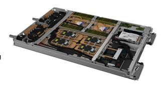
Lenovo Neptune liquid cooling reduces energy consumption by up to 40% while maintaining unprecedented compute power and density. Additionally, the SD650-N V2 is designed with a common board used by air-cooled systems, allowing you to share components across air and water-cooled systems.
