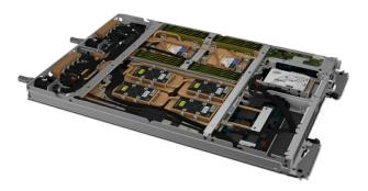
direct-to-node (DTN) liquid cooling. The SD650-N V2 brings Lenovo's Neptune DTN water-cooling technology to a GPU-based system, including four board-mounted NVIDIA A100s in a 1U system, delivering up to 3 petaFLOPS of compute performance in a single rack.
