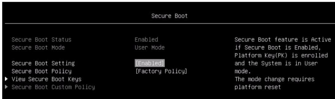
Figure 1 Enable Secure boot
