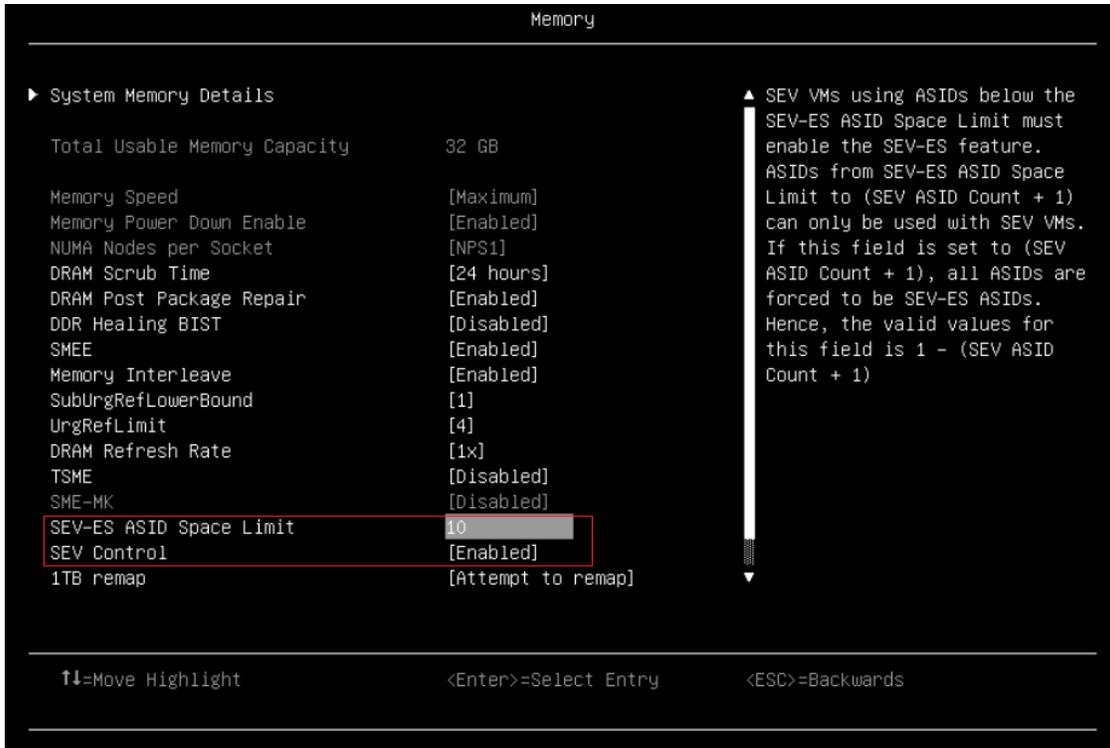
Figure 4. Enable SEV and configure SEV-ES ASID Space Limit via UEFI Settings on SR665 V3
