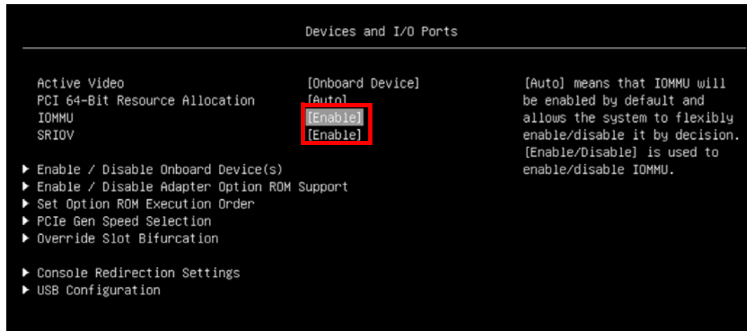
Figure 32 Enabling VT-d and SRIOV in System Setup (AMD processors)
