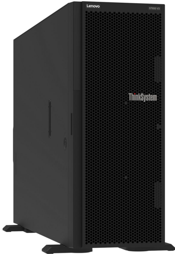
Figure 13. Lockable front security door
