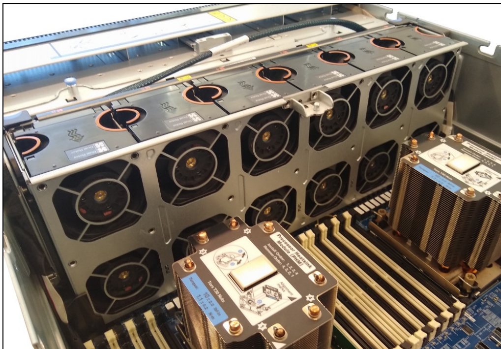
Figure 12. SR860 V3 cooling fan modules
