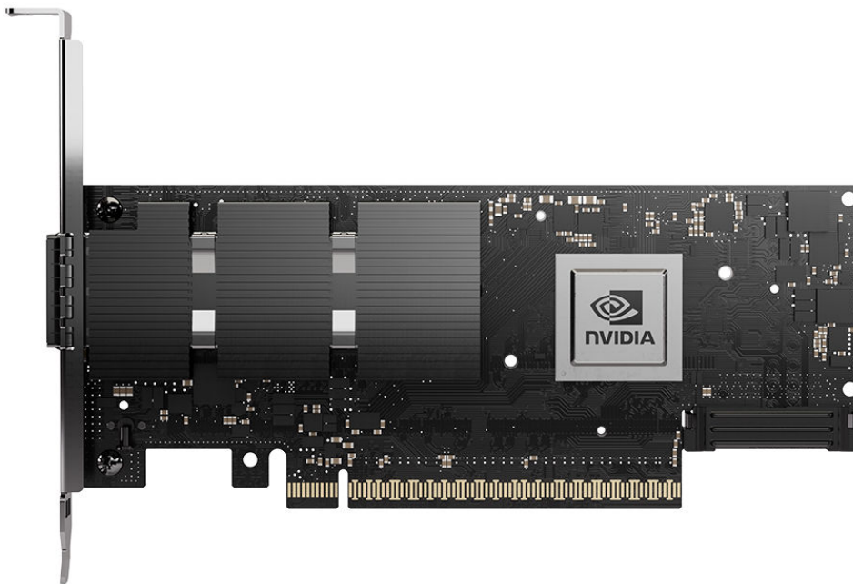
Figure 1. ThinkSystem NVIDIA ConnectX-7 NDR OSFP400 1-Port PCIe Gen5 x16 InfiniBand Adapter (4XC7A80289)
