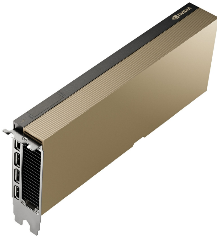
Figure 1. ThinkSystem NVIDIA L40 48GB PCIe Gen4 Passive GPU
