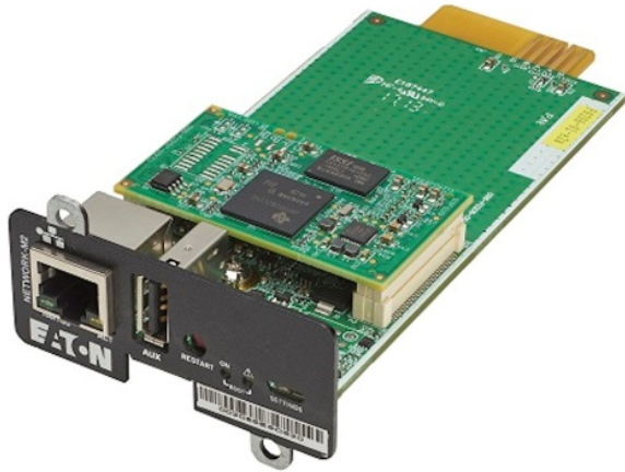
Figure 2. UPS Network Management Card
