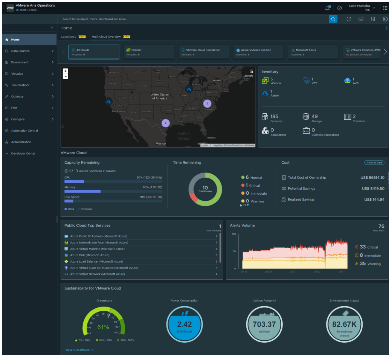
Figure 17: VMware Aria Operations home page with the new Sustainability widget showing Greenscore, Power Consumption, Carbon Footprint, and Environment Impact.
