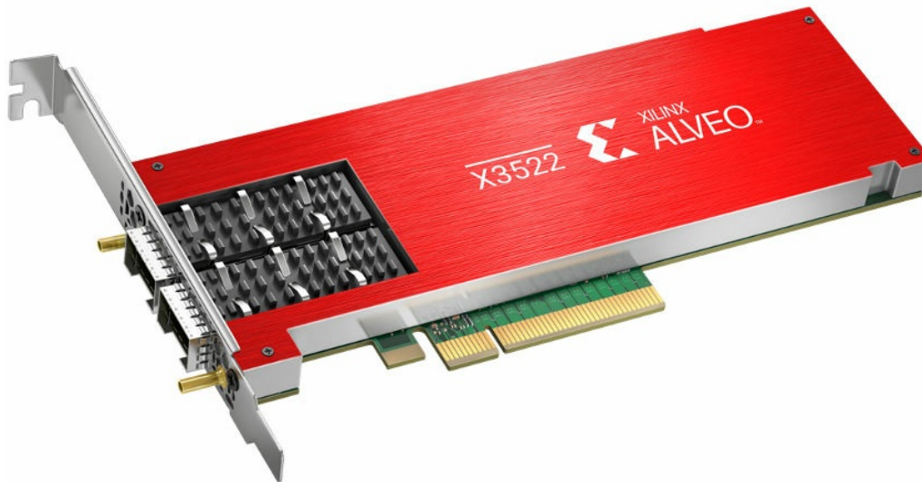
Figure 1. ThinkSystem AMD X3522 10/25GbE DSFP28 2-Port PCIe Ethernet Adapter (Low Latency)
