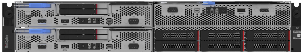
Figure 4. Front View - SD530 V3 Nodes and SD550 V3 Node installed in D3 Chassis
