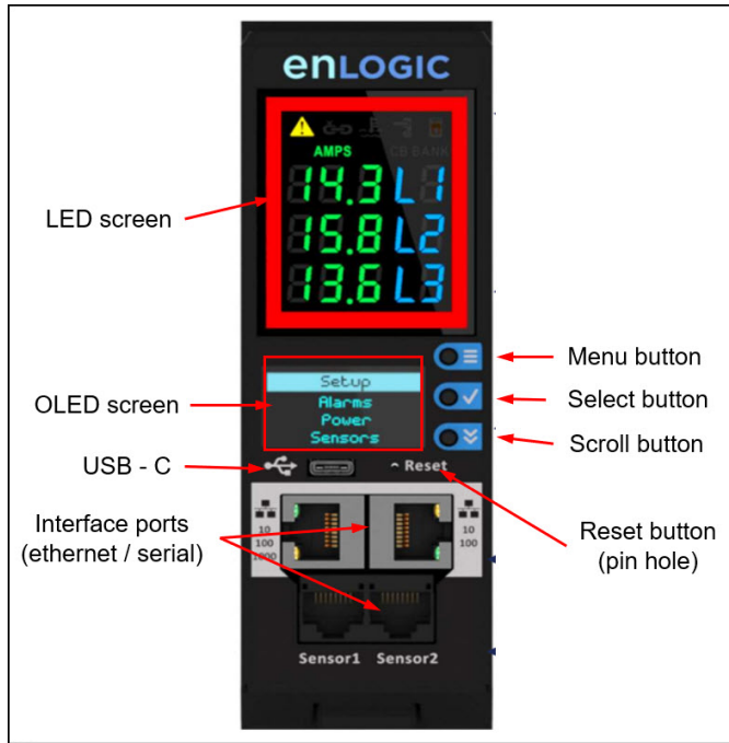
Figure 5. Interface of the Network Management Controller
