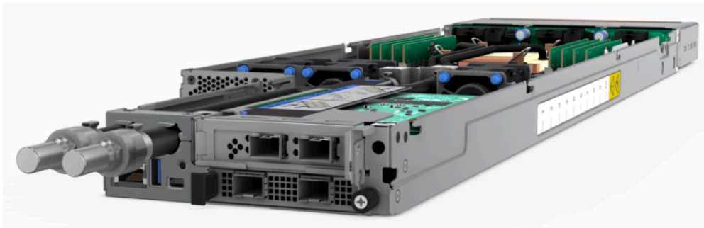
Figure 7. Rear – ThinkSystem SD535 V3 (water cooled)
