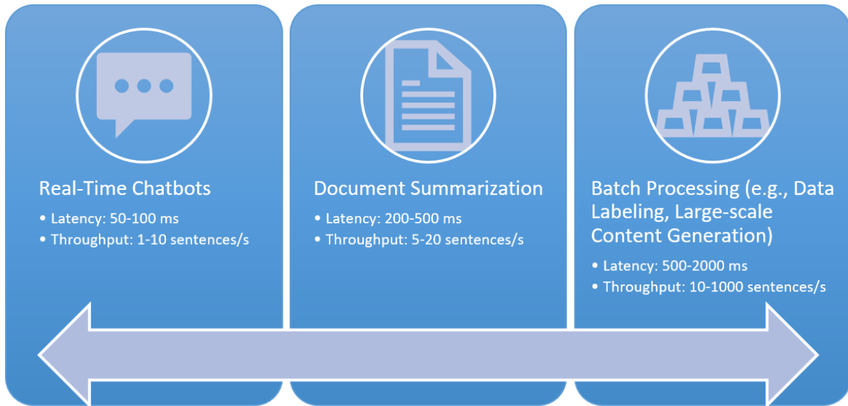
Figure 1. Common applications of large language models have varying latency and throughput requirements, from near-instantaneous chatbots to offline, mass data processing
