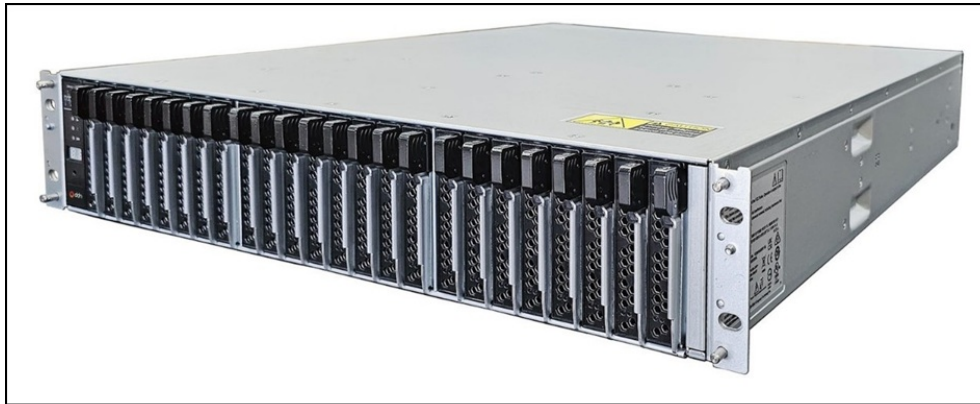
Figure 10. The DSSG - QLC enclosure unit front view
