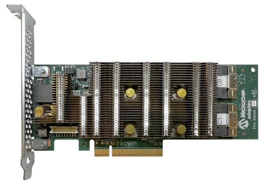
Figure 2. ThinkSystem RAID 9450-16i 8GB Flash PCIe Gen4 24Gb Adapter
