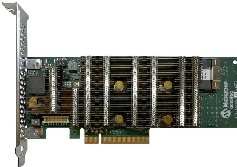
Figure 1. ThinkSystem RAID 9450-8i 4GB Flash PCIe Gen4 24Gb Adapter
