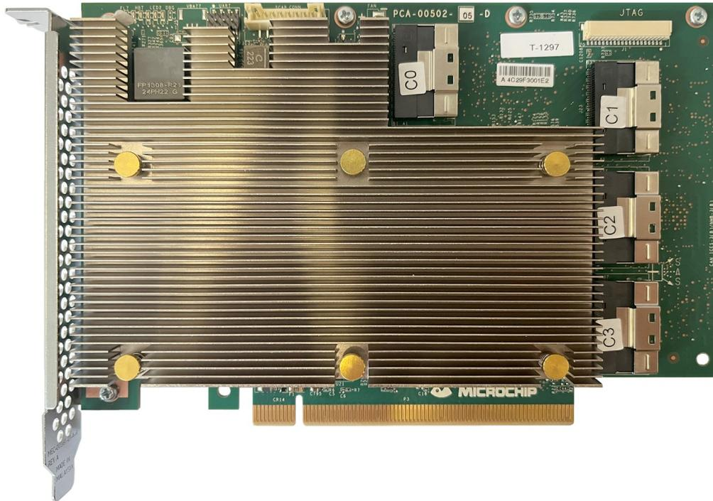
Figure 3. ThinkSystem RAID 9450-32i 8GB Flash PCIe Gen4 24Gb Adapter
