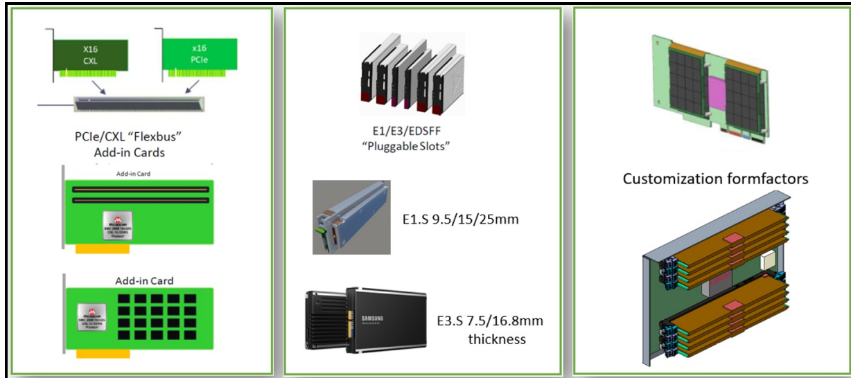
Figure 5. Several CXL memory device form factor implementations
