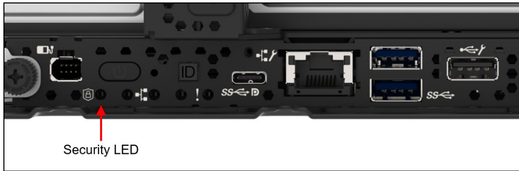
Figure 18. SE455 V3 ThinkShield Security LED
