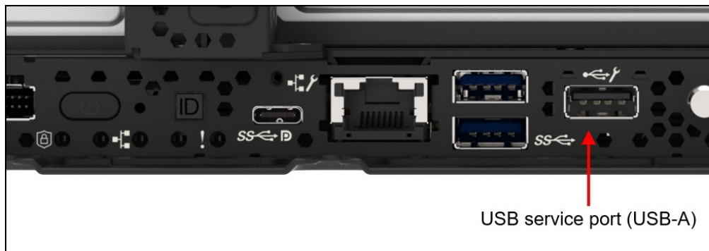
Figure 27. SE455 V3 dedicated service USB Type-A port
