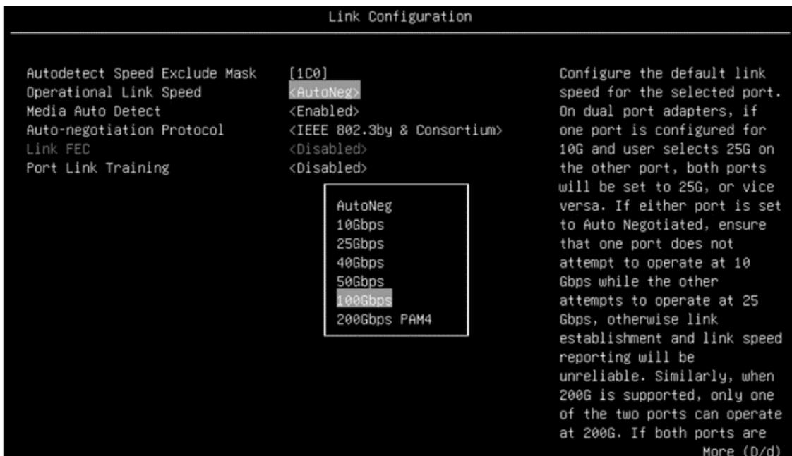
Figure 2. Operational Link Speed setting
