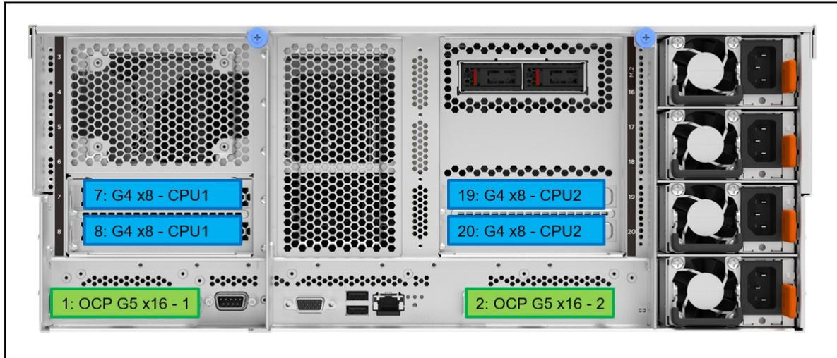
Figure 17. Slot configuration with 4x Gen4 slots
