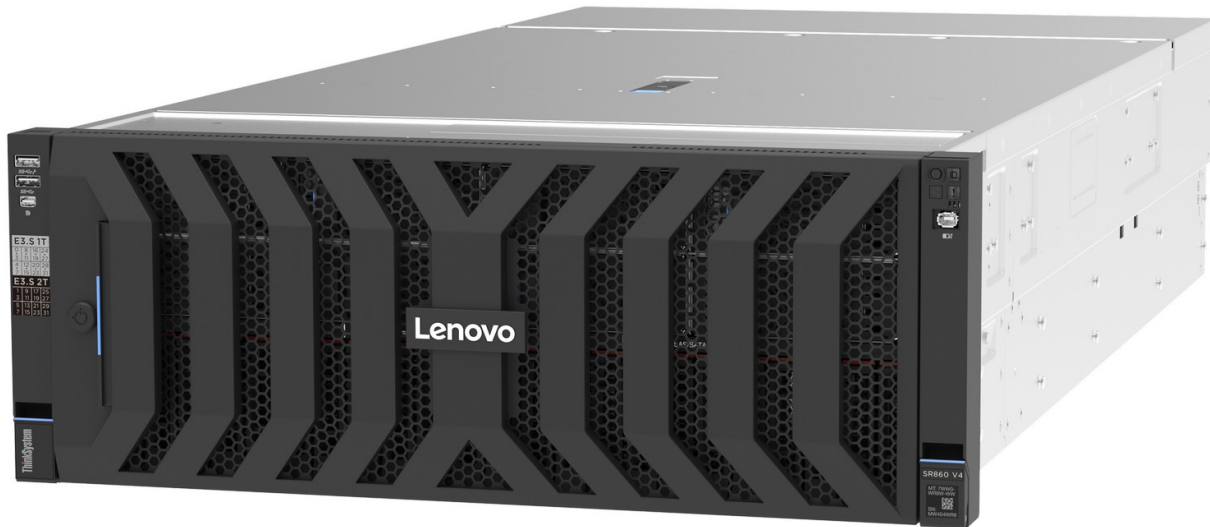
Figure 2. Lenovo ThinkSystem SR860 V4 with optional security bezel
